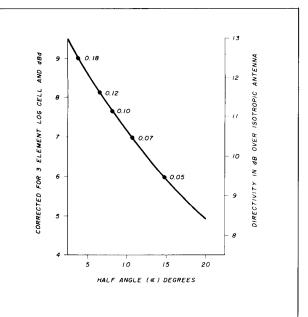
fig. 2. Extension and modification of Isbell's fig. 14.4 [Curve for  $\tau = 0.95$  only with approximate sigmas ( $\sigma$ ).]
