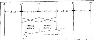
fig. 3. Log-Yagi consisting of cell ( $\ell 1$ ,  $\ell 2$ , and  $\ell 3$ ) and up to three parasitic elements.
